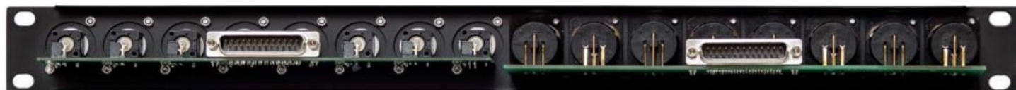
DIP-100B75 Four (4) XLR Male Output, Four (4) XLR Female Input, and Eight (8) 75 Ohm BNC Input and Output Connectors, AES Standard Digital Audio Interface, Rear View
