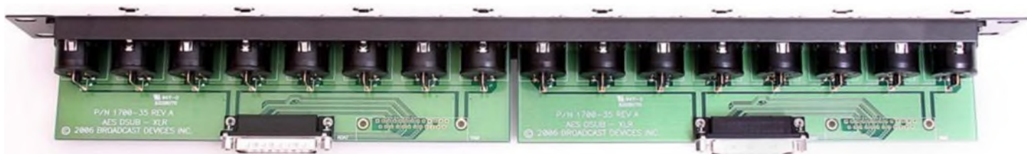
DIP-100 Eight (8) XLR Male Output and Eight (8) XLR Female Input Connectors, AES Standard Digital Audio Interface, Top View
